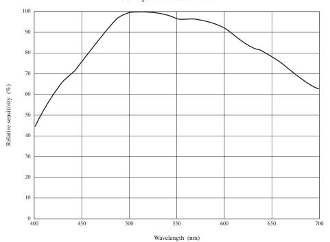
CCD spectral characteristics
